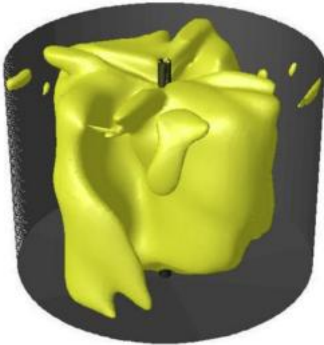
Iso-contour of axial velocity \geq particle terminal velocity
